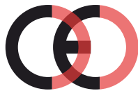
False CE Mark (too close)
